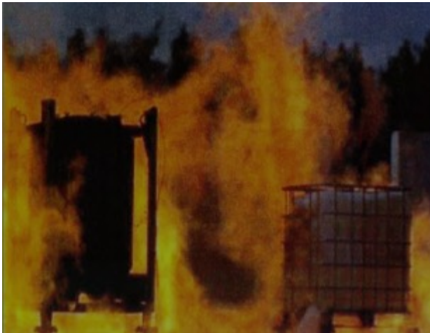
Stainless Steel and Plastic IBC during the fire test
