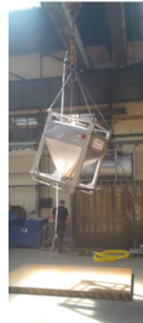
Lifting and dropping of the IBC
