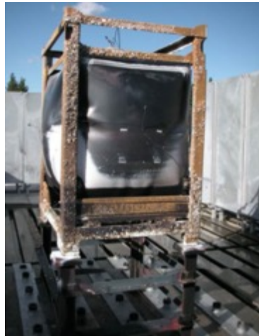
Stainless Steel IBC after the fire test
